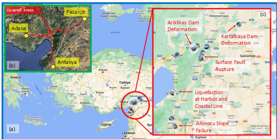
Fig. 5 Plan-view of the geotechnical reconnaissance and covered areas
