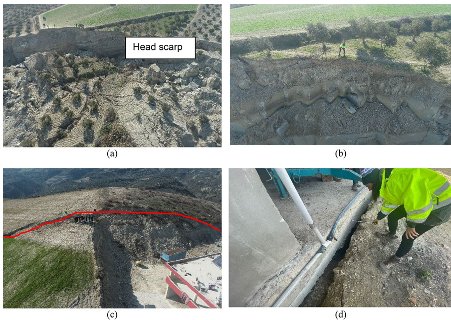
Fig. 12 Landslide at an olive farm near Turkey-Syria border (Altinozu, Hatay): a main crack (bird's-eye view) at \sim 36^{\circ}09'42.41''\text{N}/36^{\circ}13'13.40''\text{E} ; b main crack—near-front view of the crack; c potential landslide origin and tension cracks at 36^{\circ}09'28.18''\text{N}/36^{\circ}13'00.65''\text{E} d displaced single family home in Tepehan village
